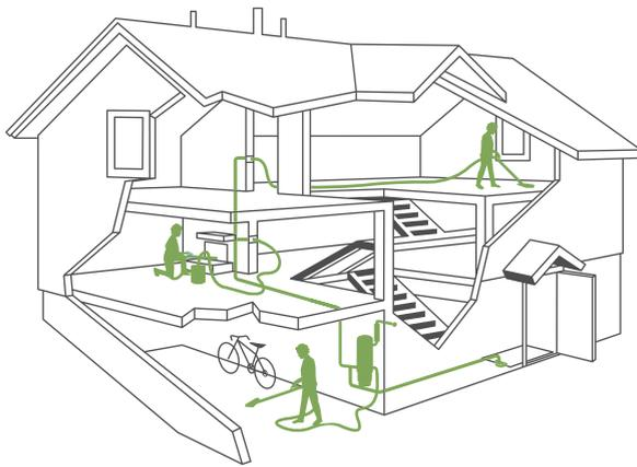
Central vacuum tubing installed through interior walls, attic, basement and crawlspaces connects vacuum inlets to the power unit/collection canister. Each strategically located inlet lets you vacuum approximately 700-800 square feet.
